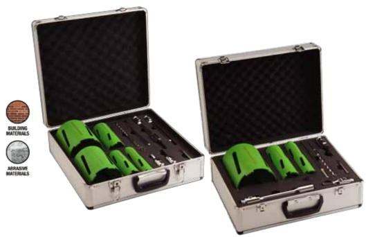
**DESCRIPTION:** The SiteTuff range of dry core drills are designed for use on the most common UK construction materials, including facing bricks and concrete blocks. The counter clockwise spiral on the core body is designed to assist in the dispersal of debris whilst drilling, helping to reduce the risk of the core jamming in the hole.
